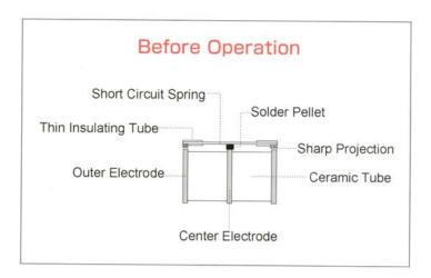
When prolonged discharge operation causes the temperature of the Gas Tube Arrester to rise to the melting point of the solder pellet, the short circuit spring moves closer to the Gas Tube Arrester and its tension forces the projections through the thin insulation making contact with both Gas Tube Arrester outer electrodes. This process permanently short-circuits all three electrodes creating a low resistance path to ground that will conduct the fault current without generating significant heat.
