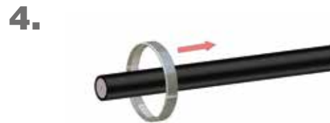
Place counter ring (1) on cable
