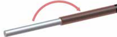
Fold back shield braid over jacket
