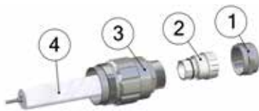
Remove cap (1) and take out sealing insert (2) from housing (3)
