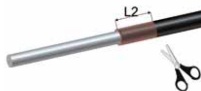
Cut shield braid roughly about 30 mm (=L2) ⚠ Carefully remove shield parts. Loose shield parts can cause electrical break down
