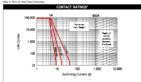
Based on extrapolated data. Since each application is unique, user is encouraged to verify rating in actual application. The load terminals should always be connected as follows: Common Contact (A2) positive; Other Contact negative.
