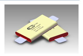
Although similar in many respects to the XKH line, the XKM SERIES is specifically designed to provide a lower profile rather than small footprint. In an effort to maintain a minimal body thickness, all XKM Series capacitors are manufactured using only a single capacitor section (winding).
