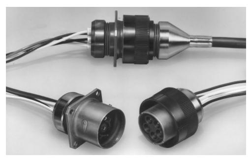
AMP 5-Pin Metal Shell Connectors are designed for high voltage circuits, especially in critical applications and harsh environments, such as shipboard applications. The connector is exceptionally lightweight and compact and can be used within a temperature range of -67°F to +257°F [-55°C to +125°C].
