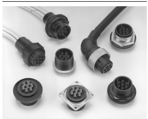
AMP 7-Pin Miniature Circular Connectors, when properly assembled and mated, safely carry 15 KVDC (pin-to-pin and pin-toground) through a full range of military environmental requirements. The connectors can carry a continuous current of 7.5 amperes per line when terminated to 20 AWG wire. The receptacle
